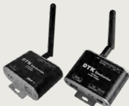
**Zigbee to USB converter & Zigbee to RS485**
